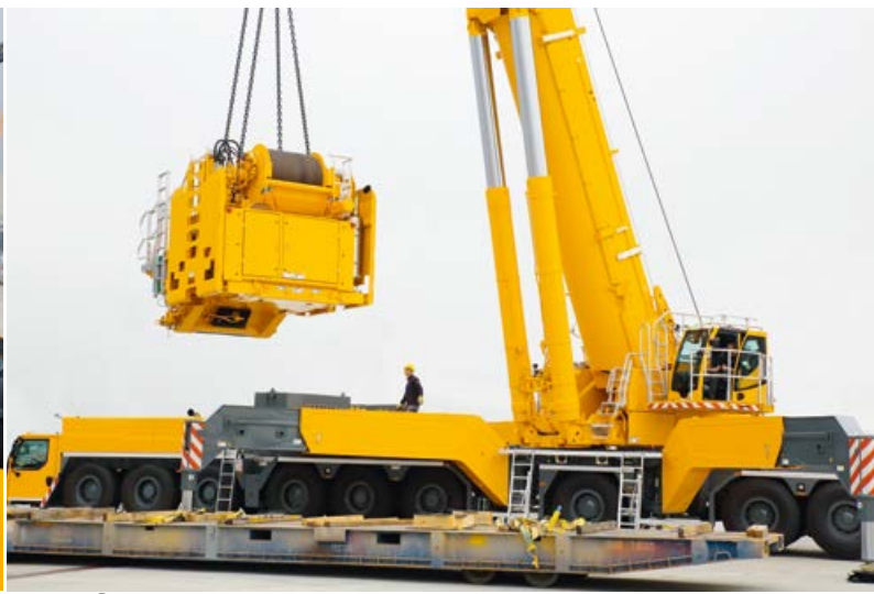
⑥ Self-assembly counterweight frame with drive assembly
