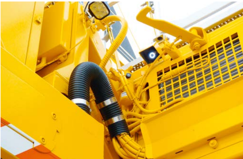
Camera monitoring of the rear of the crane cab
