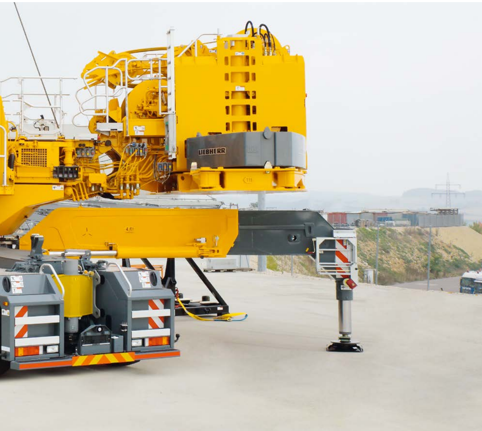
⑦ Cylinder of the counterweight frame fixed to the ballast ground plate
