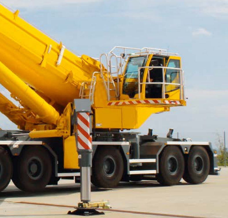
③ Self-assembly of the rear outriggers
