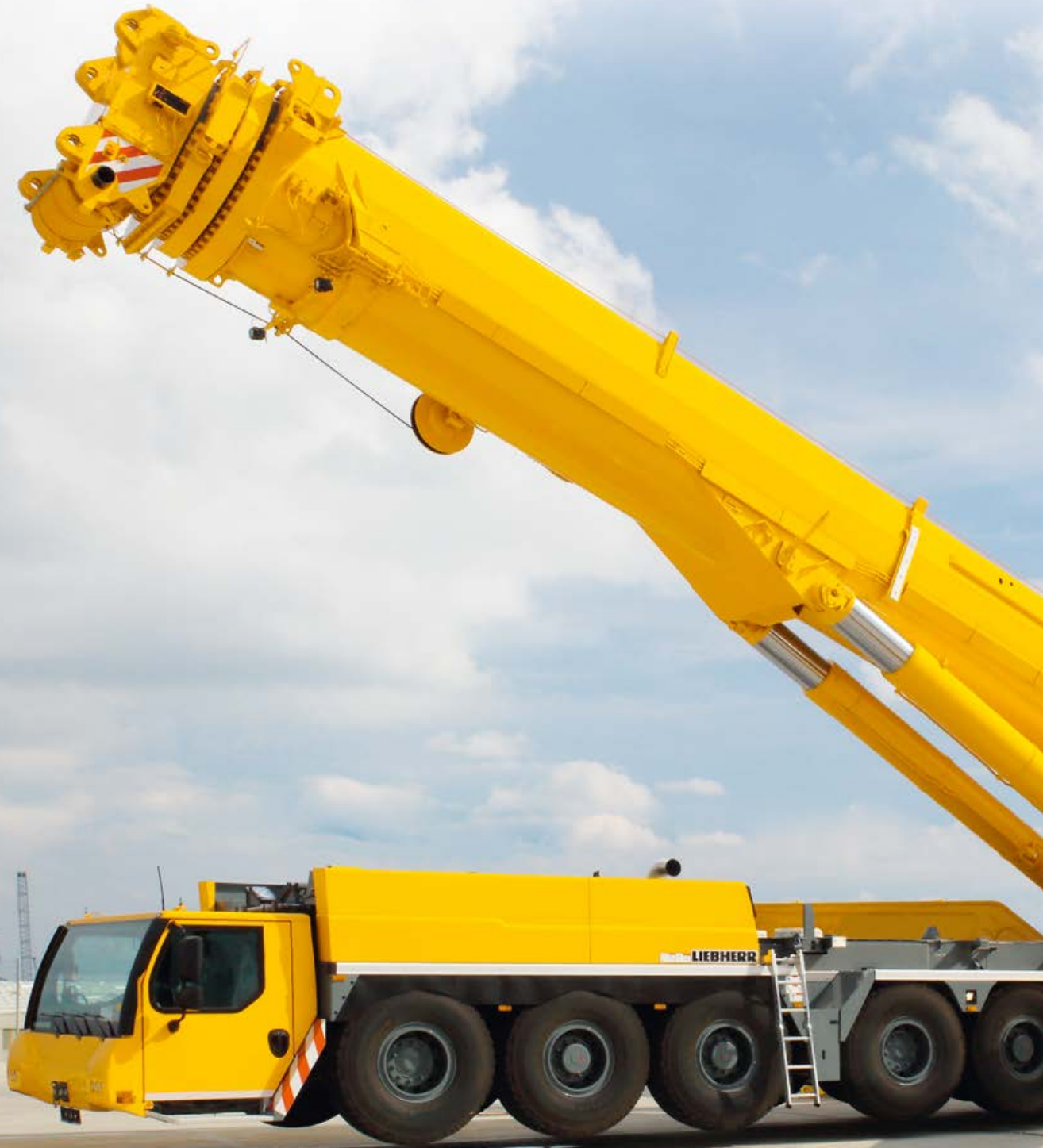
① LTM 1750-9.1 supported on the front outriggers
