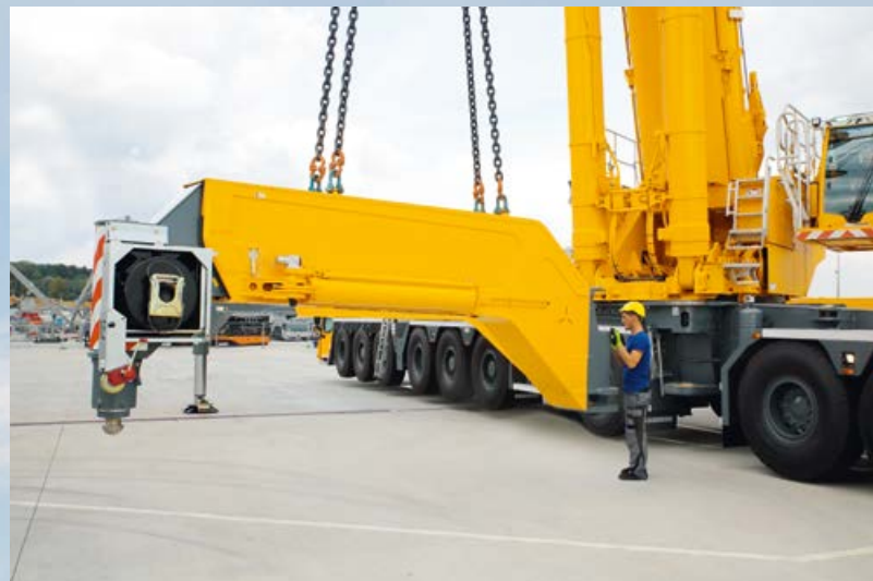
③ Self-assembly of the rear outriggers
