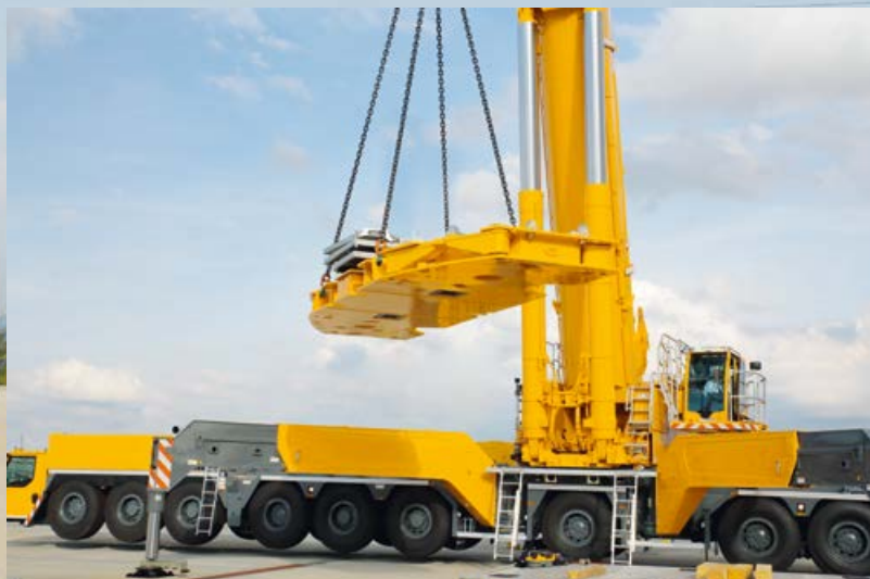
④ Self-assembly counterweight
