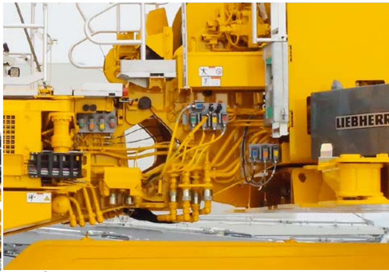
⑧ Connecting hydraulic and electric quick couplings
